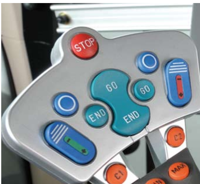
Operating buttons for 3rd and 4th auxiliary hydraulic control units
