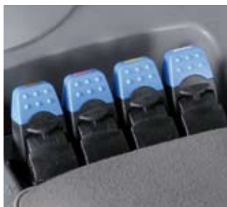
Controls for auxiliary hydraulic control units
