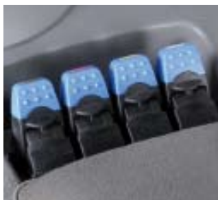
Controls for auxiliary hydraulic control units
