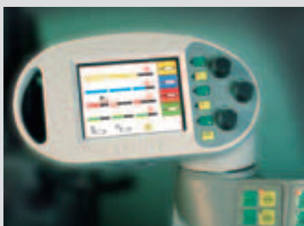
Fine adjustments to the valve functions can be made on the Varioterminal. For example, you can control the flow rate precisely and easily using the rotary controls and function keys.
