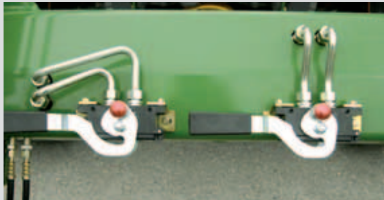
The optional third and fourth hydraulic circuit for attachment actuation can also be fitted with multi-couplers upon request.
