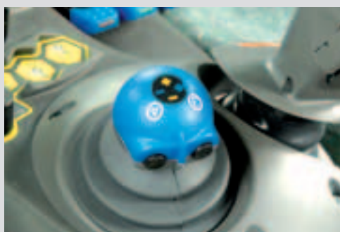
The standard-equipped crossgate lever controls the front loader very precisely via two control valves. When working with a silage or bale grab, the third hydraulic circuit (optional) can be actuated with a push-button on the crossgate lever.
